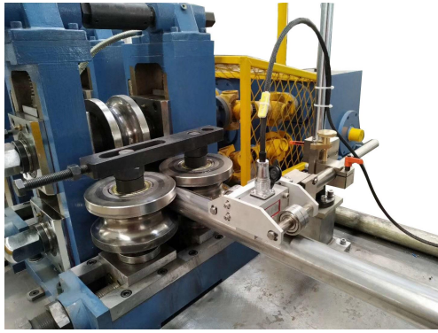
Weld Seam Inspection Round Pipe
