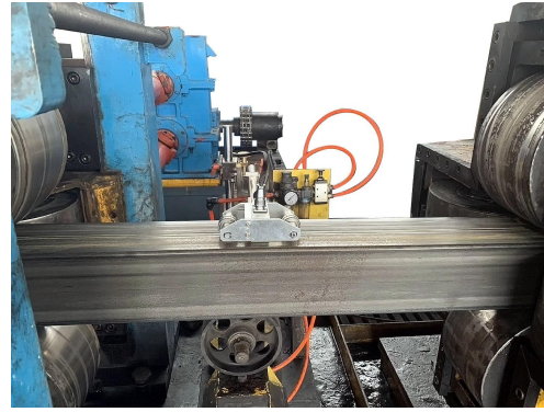
Weld Seam Inspection of Square Tube
